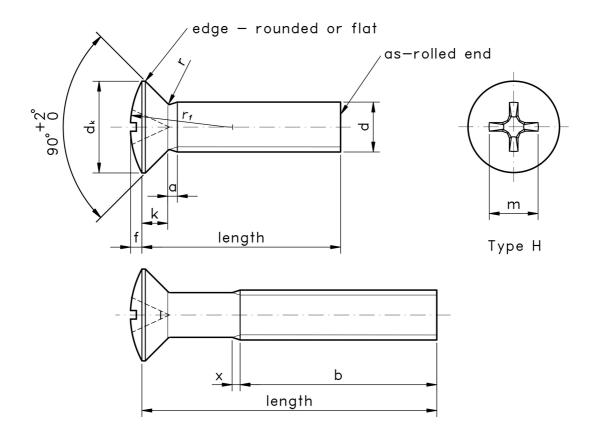
Figure 1: Phillips Raised Countersunk Head Machine Screw
