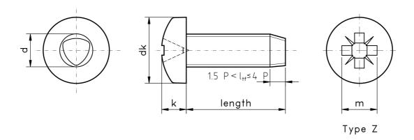
Figure 1: Pozi Pan Thread Rolling Screw
