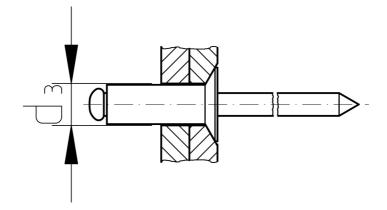
Table 4/Figure 2: Joint hole diameter according to DIN 7337
